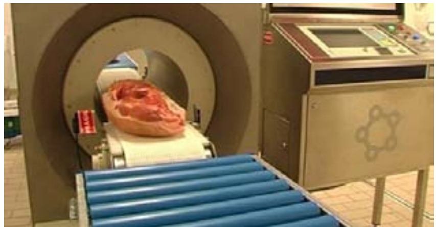
Fig.1: Ham-grading system (JMP Ingenieros, S.L., Sotés, La Rioja, Spain).
